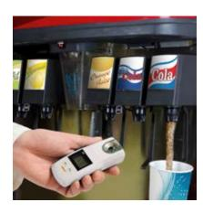
The concentration of sugar, important quality characteristic for the production of wine or jam, can be determined very fast and reliable with the Brix-refractometers. This is the typical application of refractometers.
